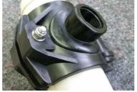
Now the clamp is closed and has to be screwed using the washer and a self-locking nut (10 Nm). The thread of the hexagon screws should be lubricated beforehand to avoid seizing.
